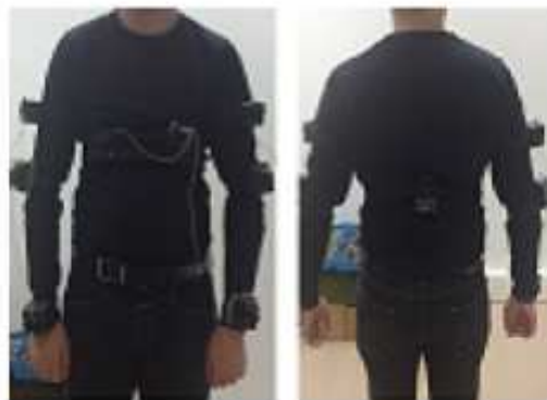
Figure 3.7: On-body network deployment scenario for MoCap experiments during the 1 st measurement campaign.
