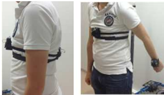
Figure 3.4: Experimental Scenarios 1.5 (left), 1.6 (right): On-body ranging over static chest-back and chest-wrist links respectively, under systematic NLOS conditions.
