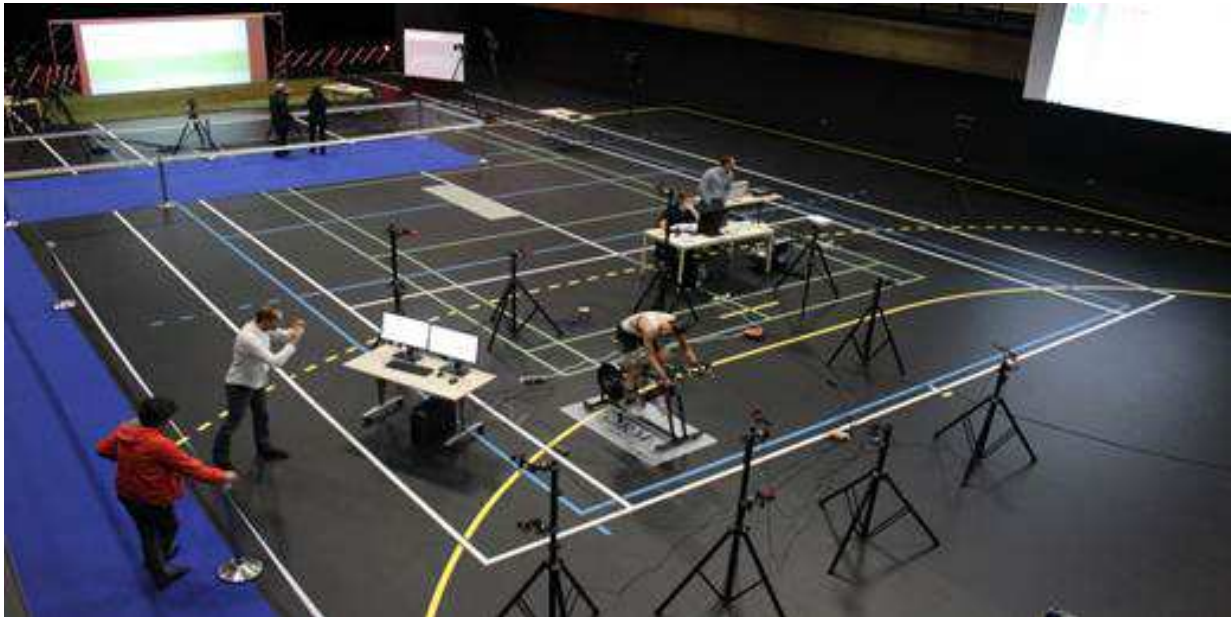
Figure 2.6: “Vicon” optical acquisition & tracking system (example of capture), delivering the reference location information for WBAN-based MoCap and navigation applications in the second measurement campaign.
