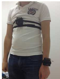
Figure 3.1: Experimental Scenario 1.1: On-body ranging over a static chest-wrist link in direct LOS visibility.
