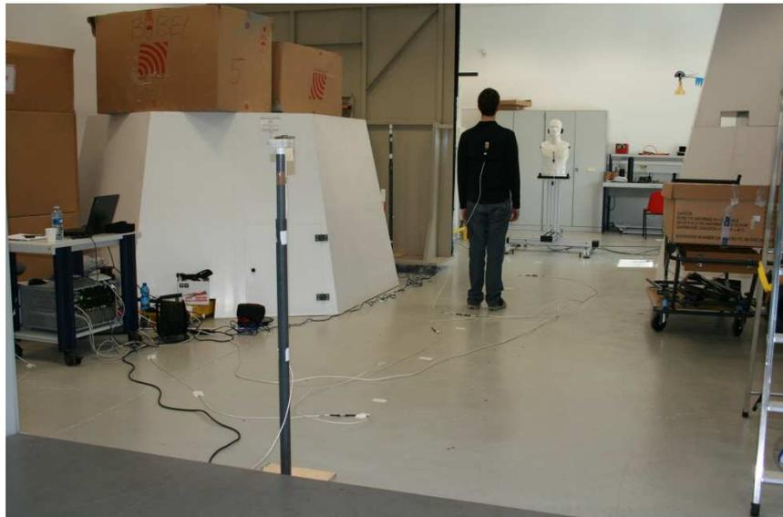
Figure 78 : Photography of a WBAN measurement in a cooperative scenario
