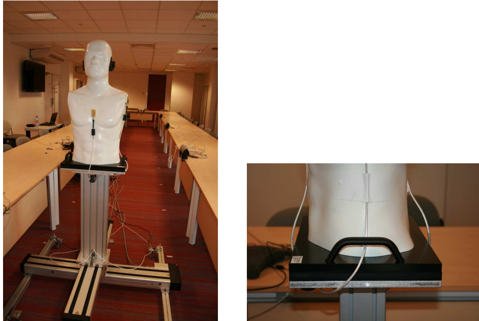
Figure 2 : Pictures of the realized mechanical mount for the phantom placement on the (X, Y) positioner
