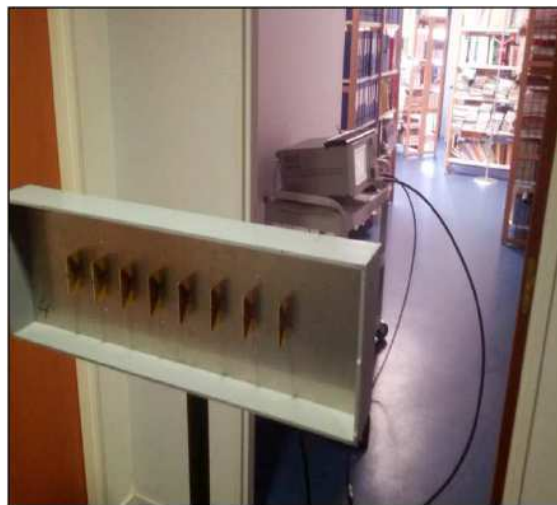
Figure 28 : Rx antenna is the 5th element from the left
