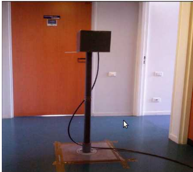
Figure 27 : The Tx antenna on site - notice the hard fixation on the ground to avoid undesirable displacement by moving people
