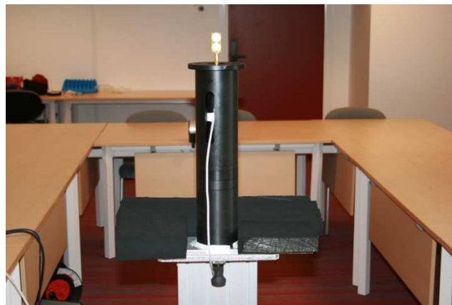
Figure 7 : Picture of the Rx antenna placed on a mast to perform the benchmark measurements
