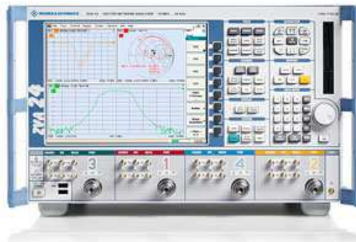
Figure 37: Rohde & Schwarz ZVA 24 Vector Analyzer
